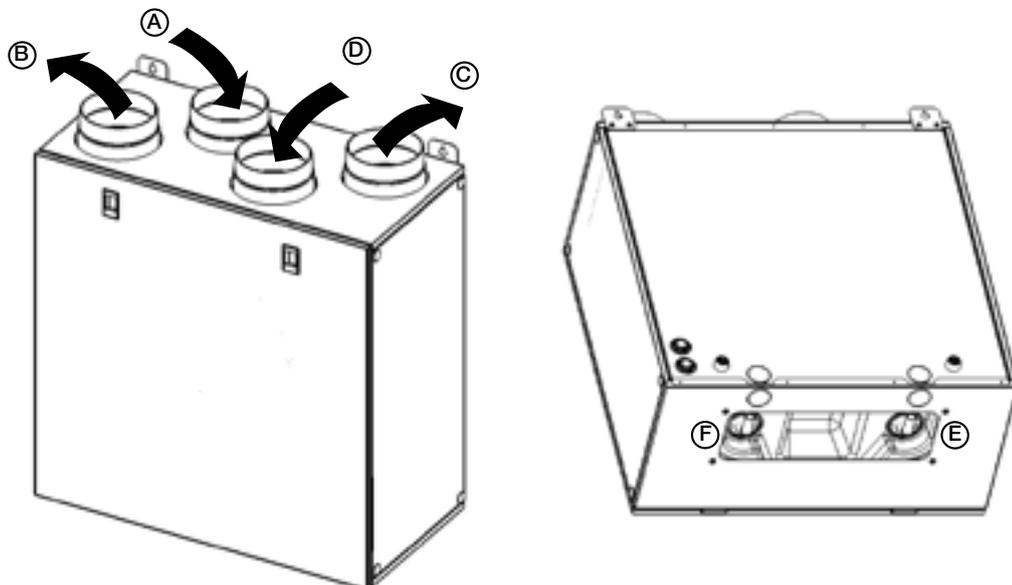
**Fig. 3.b** Connections in RIGHT orientation
