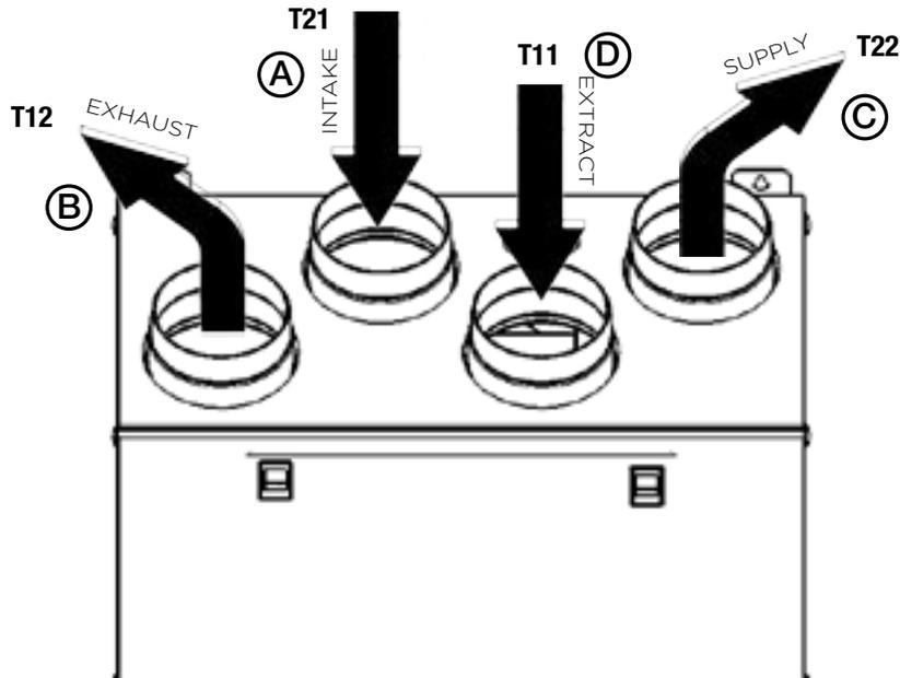
**Fig. 7.a Temperature probes in LEFT orientation**
