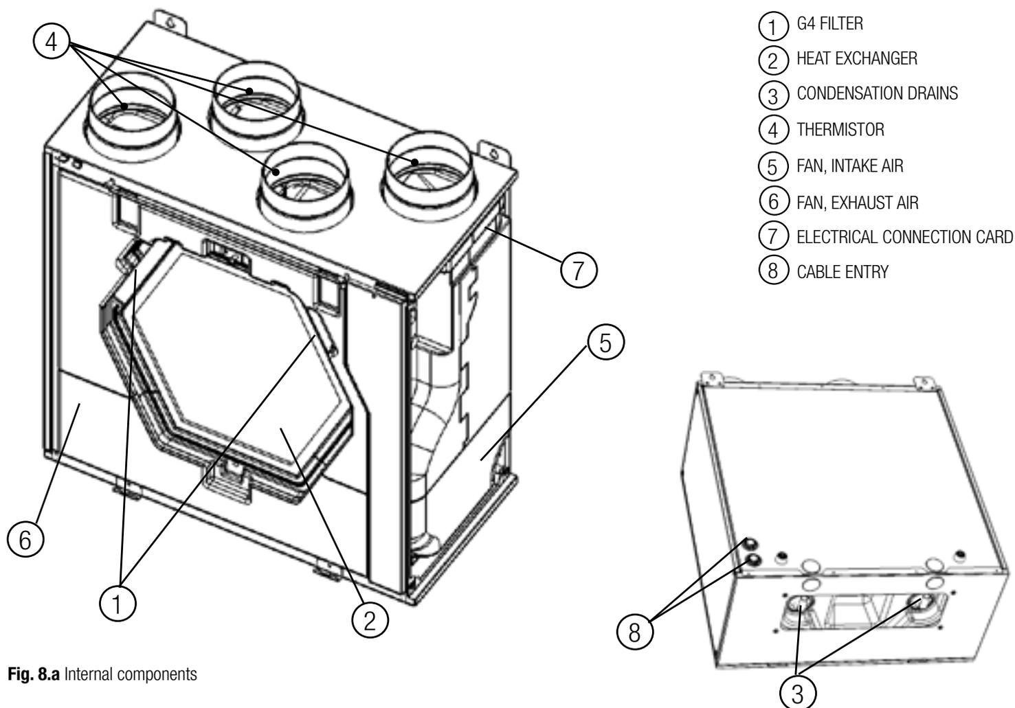
**Fig. 8.a** Internal components
