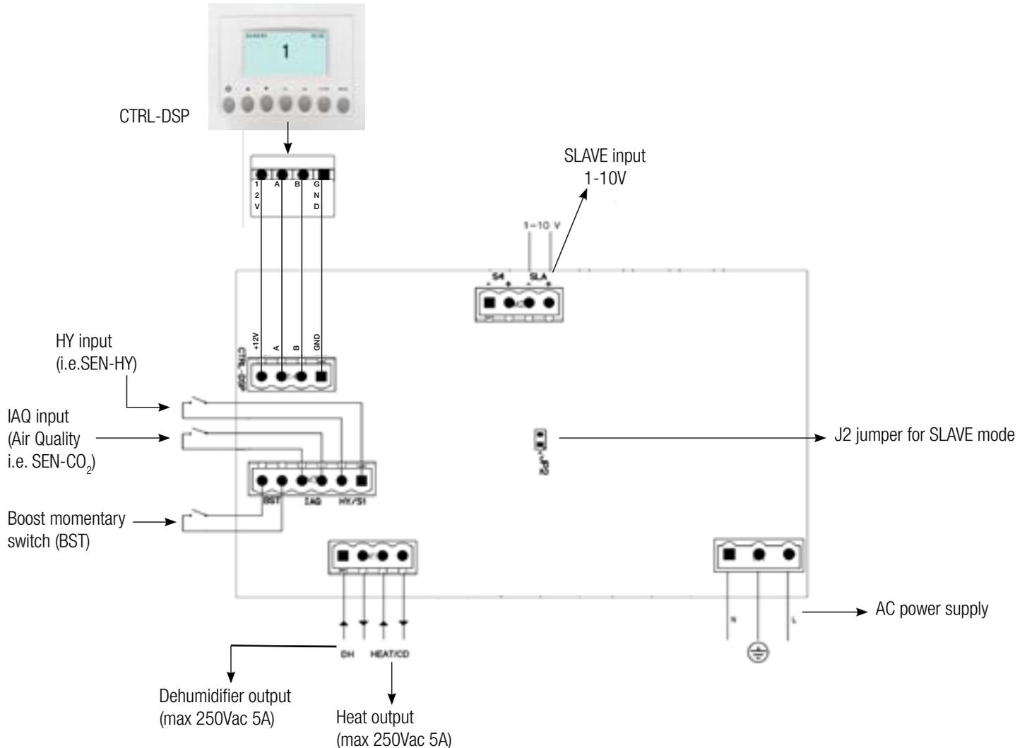
Fig. 5.1 Electrical connections on the motherboard fitted in the terminal box.
